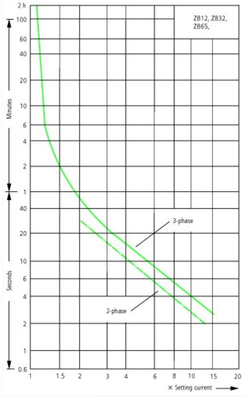
These tripping characteristics are mean values of the spreads at 20 °C ambient air temperature in a cold state. Tripping time depends on response current.
